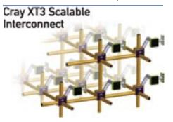
Interconnect router – The router in the Cray SeaStar chip provides six high-speed network links which connect to six neighbors in the 3D torus. The peak bidirectional bandwidth of each link is 7.6 GB/s with a sustained bandwidth in excess of 4 GB/s. The router also includes reliable link protocol with error correction and retransmission.
